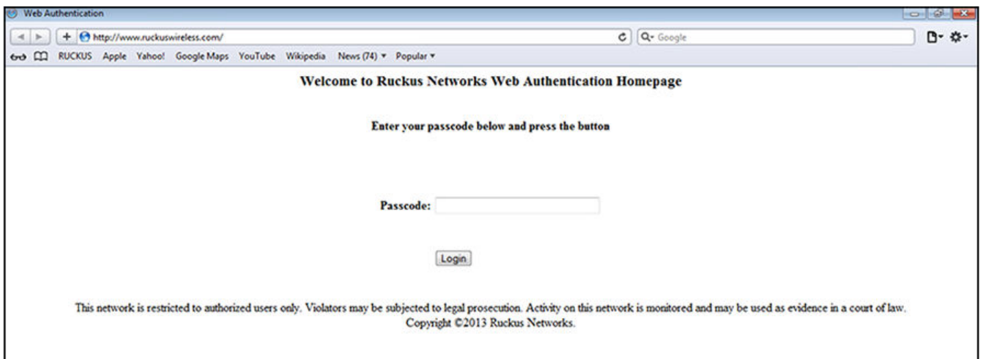
FIGURE 21 Example of Login Page When Automatic Authentication Is Disabled and Passcode Authentication Is Enabled
